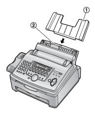
2 Pull the tension plate forward (①) and attach the paper tray cover (②), then push the tension plate back (③).
